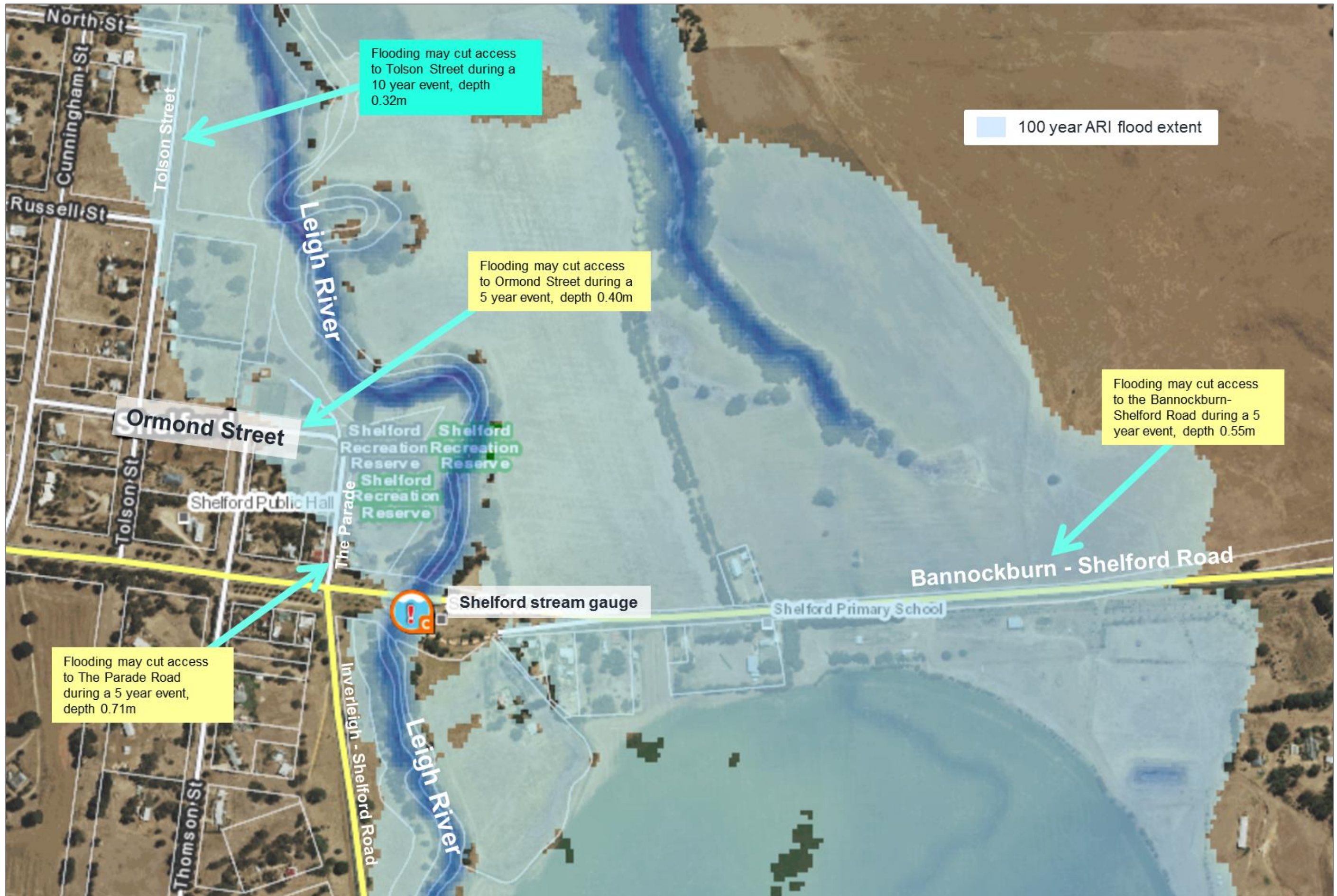
Figure 39. Shelford roads impacted by flooding with the 100 year ARI flood extent (DELWP 2016).
