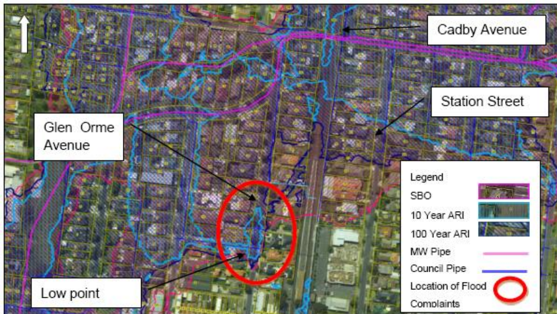
Figure A2-2: Flooding from the Koornang Road Main Drain at the southern end of Glen Orme Avenue
