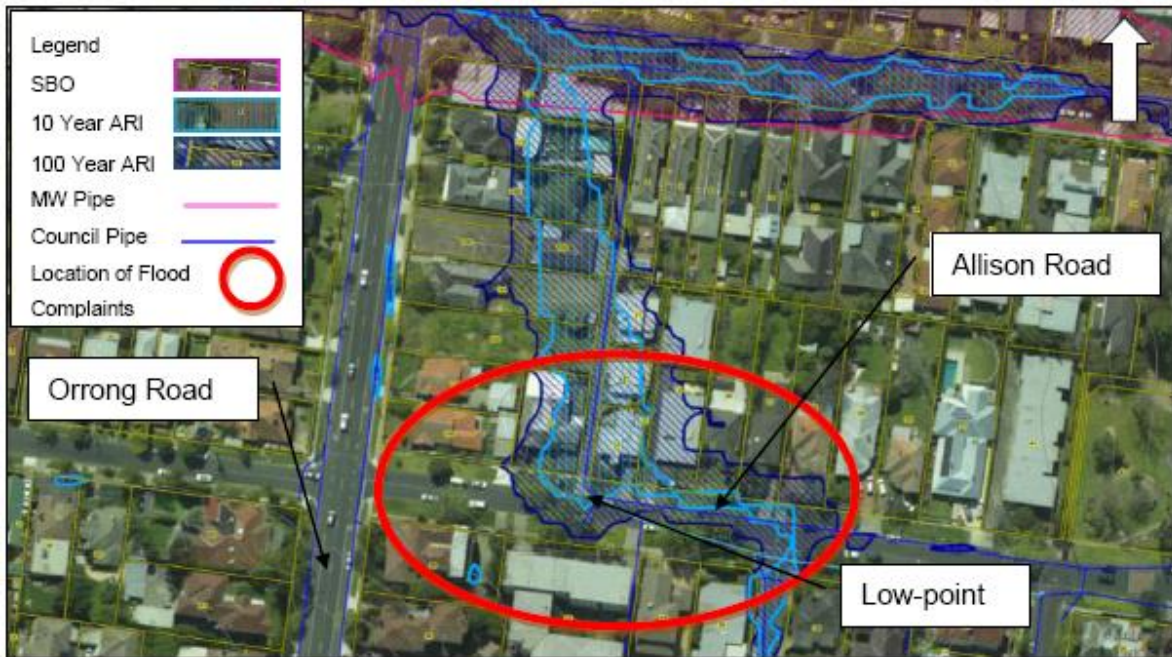
Figure A3: Flooding in Alison Road near Orrong Road
