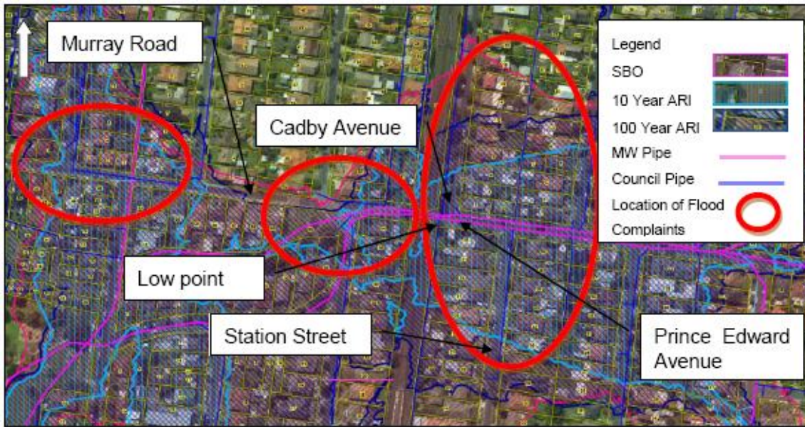
Figure A2-1: Flooding along the Koornang Road Main Drain
